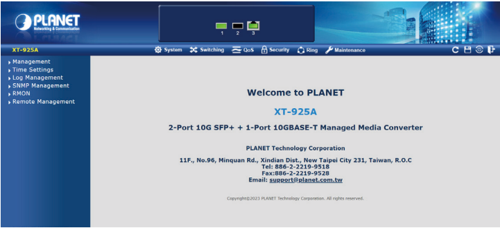
Figure 2. Web Main Screen of Managed Media Converter (Use XT-925A as a representative)
